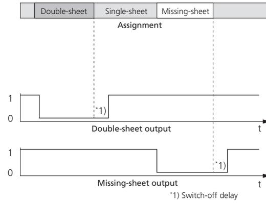
Fig. 7: dbk-4/CDI/OIM18 (Double-sheet output) and dbk-4/CDD/SIM18 Free-Run-Mode
