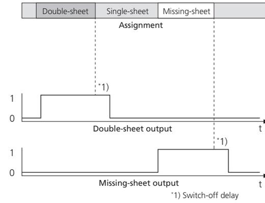
Fig. 8: dbk-4/CEE/OIM18 Free-Run-Mode
