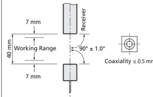
Fig. 3: Installation and working range
