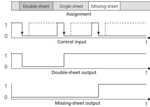
Fig. 10: dbk-4/BEE/OIM18 Trigger-Mode
