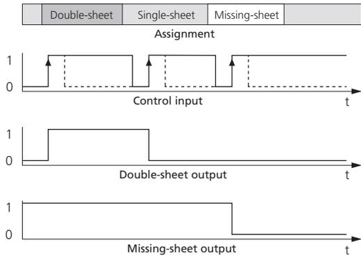
Fig. 9: dbk-4/BDD/OIM18 Trigger-Mode
