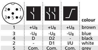
III. 3: Pin assignment with view onto sensor plug and colour coding of the microsonic connection cable
