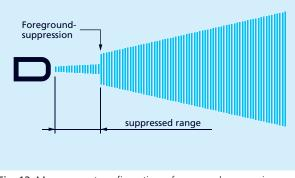
Fig. 12: Measurement configuration – foreground suppression
