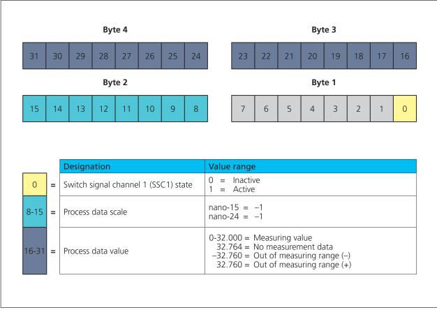
Fig. 4: Process data structure
