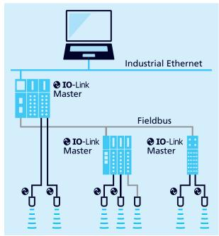
Fig. 1: Structure of an IO-Link system
