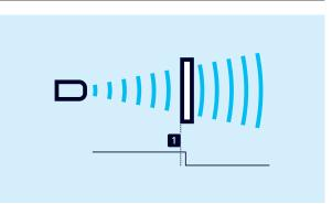
Fig. 7: Switching point (Method B), single point + set point offset
